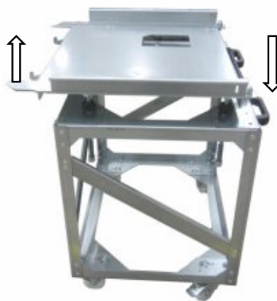
Service trolley handle fixator should be pushed down for trolley guides fixing in the guide openings of the panel
